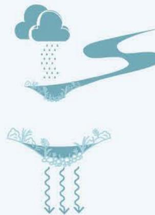
A dry creek is a retention corridor designed to receive wet weather runoff during rainy episodes.
